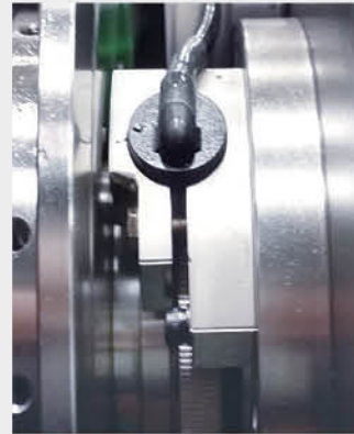
Changed spindle rotation detection sensor eliminating a cause of service issues
