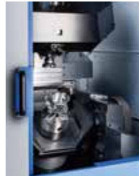
Accessibility to jig or workpiece with A-axis at -30 deg.
